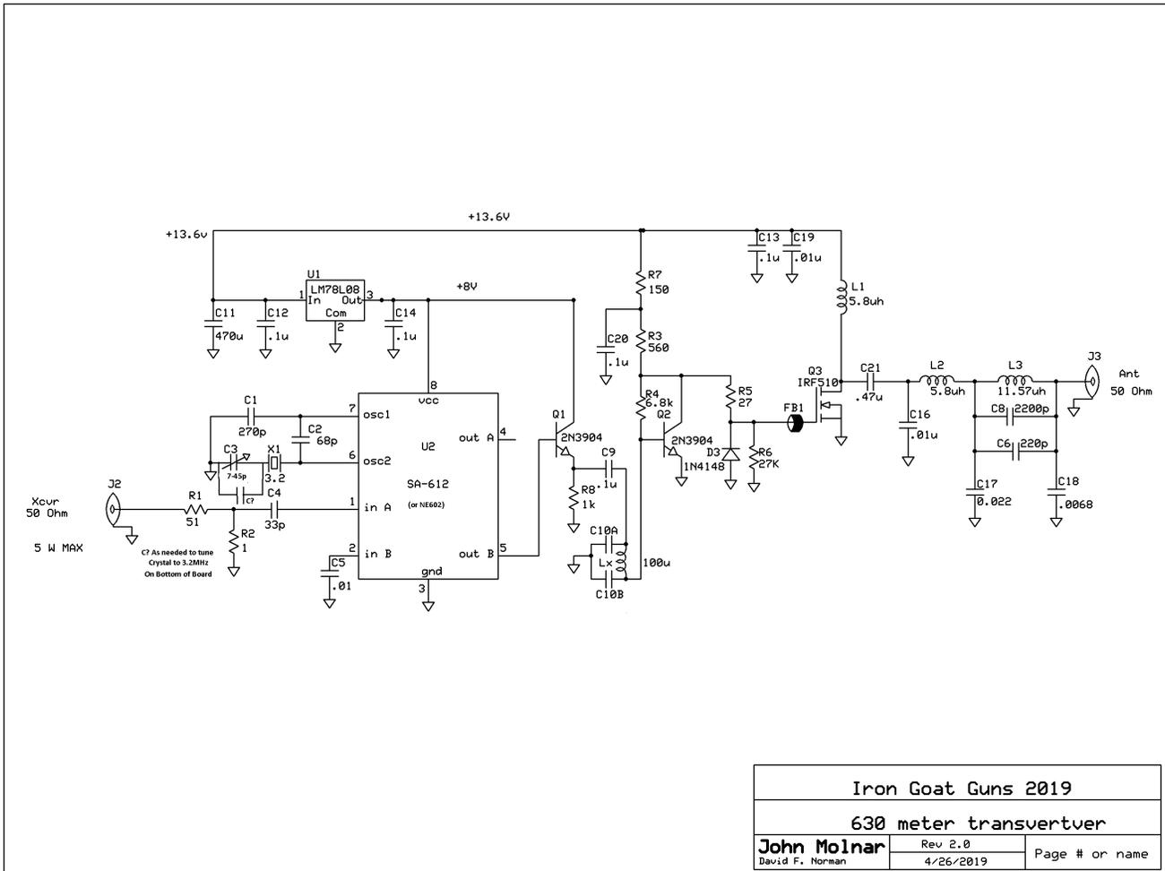
The simple schematic above shows the electrical connections of the transverter. The blank board shows the physical layout. The parts list has all of the actual components, giving a competent Amateur all he needs to know about repairing the unit should it ever become necessary. Observe the cautions listed below and you should expect years of good service until something better comes along.
